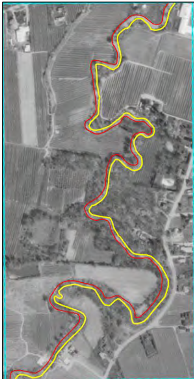
Figure 6-3: Banklines in 2000 Aerial Imagery Figure 6-4: Banklines in 2015 Aerial Imagery
