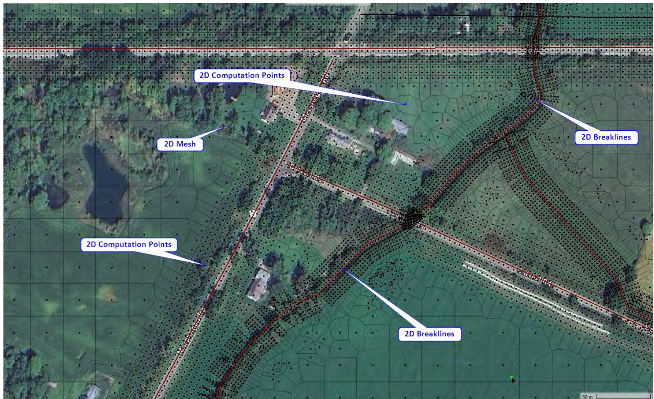
Figure 4-3. 2-D Mesh Visualization
