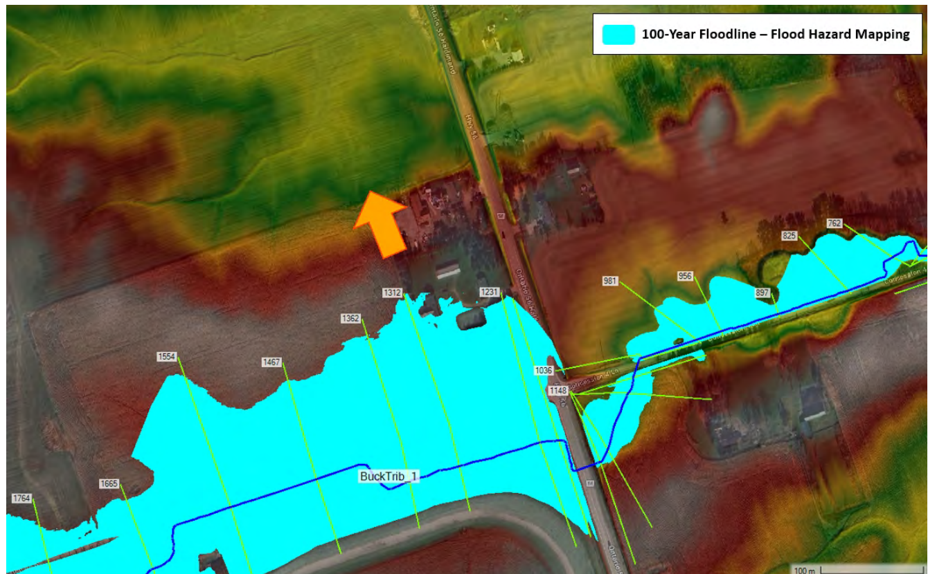
Figure 5-12. Reach BuckTrib_1 Spill to Adjacent Watercourse
