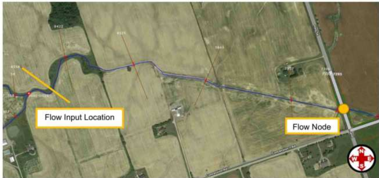
FIGURE 4.1: INCORPORATION OF FLOWS INTO HYDRAULIC MODEL
